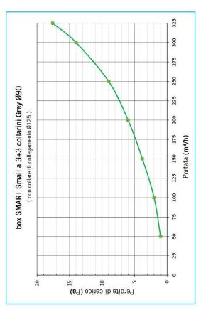
Pressure drop graphs of SMART Small boxes mod. VMSMART12\_690 (the "+ 2 collars" graphs refer to boxes with the addition of VMSMPL290 plate; in the total  $\Delta p$  (the  $\emptyset$ 125 flexible hose section is included)
